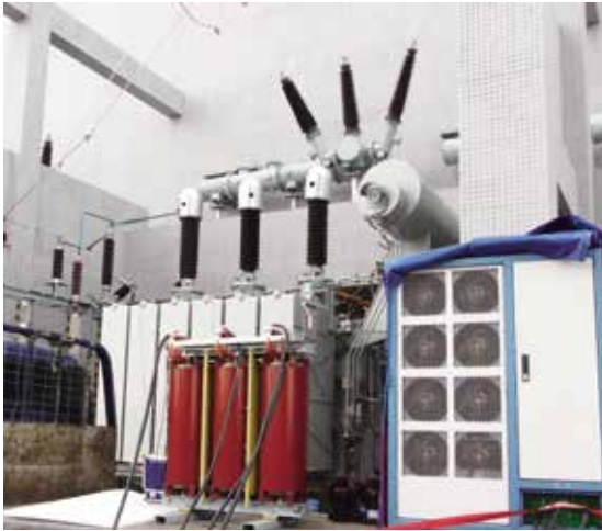
110kV 3-phase transformer simultaneous on-site test in Duishan, Xiamen, Fujian Province
